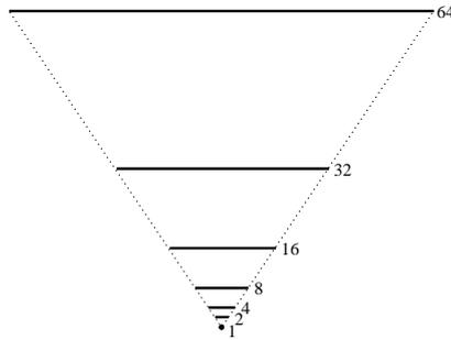
Figure 1: Side view for a mipmap for a texture of size  $64^2$
