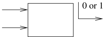
Output stuck at 0 or 1
