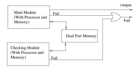
CS\_313/CS\_M13 Sect. 6 (g) 46/62 6 (g) Hardware Fault Tolerance
