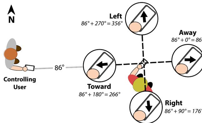
**Figure 2:** Tilt gesture directions the hotspot receives are based on the bearing between the controlling and hotspot devices. All instructions are egocentric.
