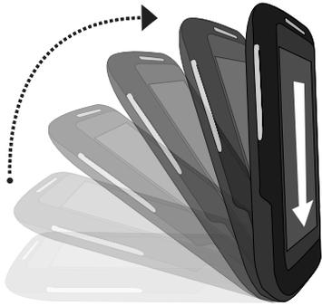
**Figure 1:** Tilting towards - sending an instruction to walk towards the controlling user. The controlling user can tilt their device backwards or forwards to make a hotspot walk towards or away, and left or right to turn left or right (not shown).
