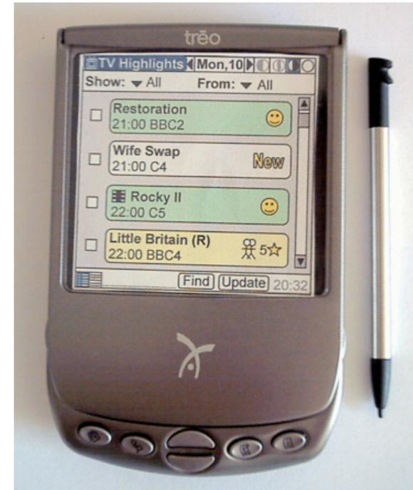
**Figure 2.** The design concept mock-up used in evaluations. Shows *TV Highlights* dialogue giving user personalized information for near future.
