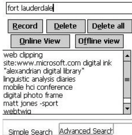
Figure 1: handheld application for query capture. User is entering a new query and a list of all previously entered queries is shown. Some of the queries (e.g. "site:www.microsoft.com digital ink") were entered using the "Advanced Search" interface.
